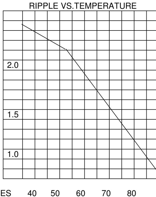
Ripple current capability depends upon case area and ESR because ripple current dissipates power in the ESR and case area determines the core temperature rise. A different capacitance from that listed in Standard Ratings Table will have a different ESR and, therefore, a different ripple current rating. The ripple capability is proportional to square root of capacitance for the same WVdc and case size.
